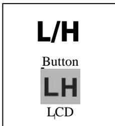
The speed can be set to low or high with the L/H button. Standard setting is H (High), press the button to switch to L (Low). Switch the scooter OFF and ON the Low / High speed shall not be remembered and automatically goes back to the standard value H (High). H or L is shown on the LCD screen to indicate which value is selected.
