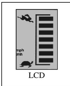
The driving speed bar is shown on the LCD screen to indicate the driving speed.
