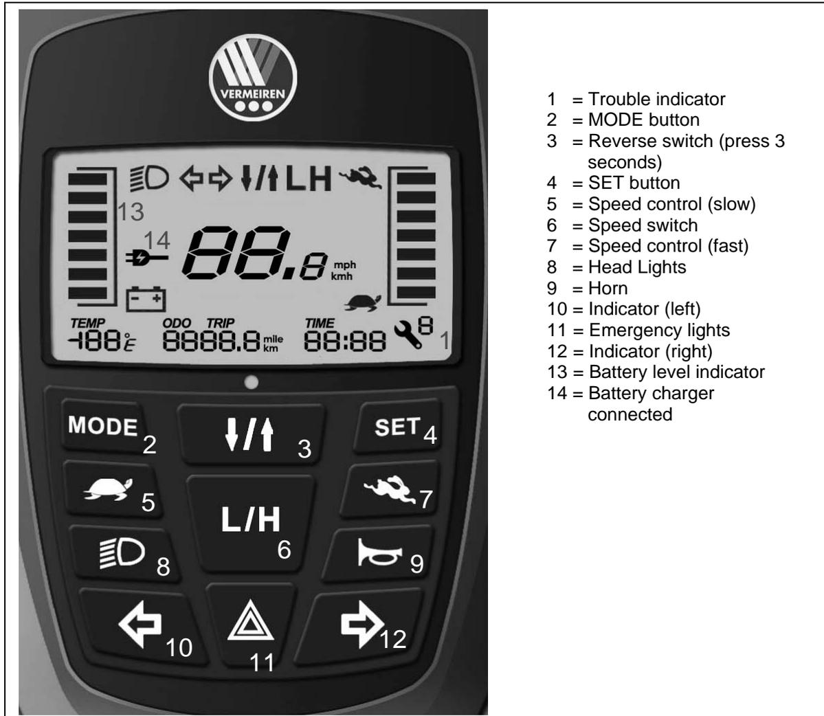
Put the ON/OFF key switch on, please wait for at least 3 seconds before you press the speed lever otherwise you have a "delay protection" alarm.
