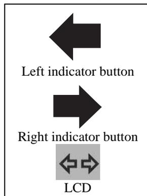
To put on the indicator lights, press the desired button (left = left indicator, right = right indicator). At the same time the button will turn green and has a sound from a horn. Press the Button again to turn the indicator off.
