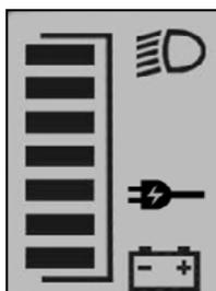
The battery charge indicator is used to indicate that your scooter power is on and provides an estimate of the remaining battery capacity.
