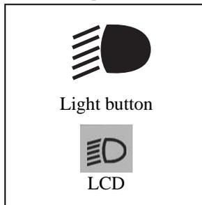
To put on the front and back lights, press the light button, button will turn green. Press again to turn the lights off. The LCD screen shown a light symbol to indicate the lights are activated.
